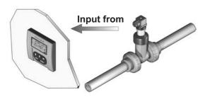
The panel mounting version consists of the monitor and the mounting bracket kit F9.KP1 with gasket for IP65 watertight panel installation. The monitor perfectly fits into a standard ¼ DIN panel cutout. The instrument and the kit can be ordered separately (code F9.20 for the monitor and code F9.KP1 for the mounting bracket) or together using the code F9.20.P1.
