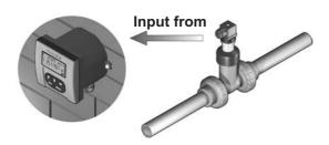
The wall mounting version consists of the monitor and the wall mounting kit.
